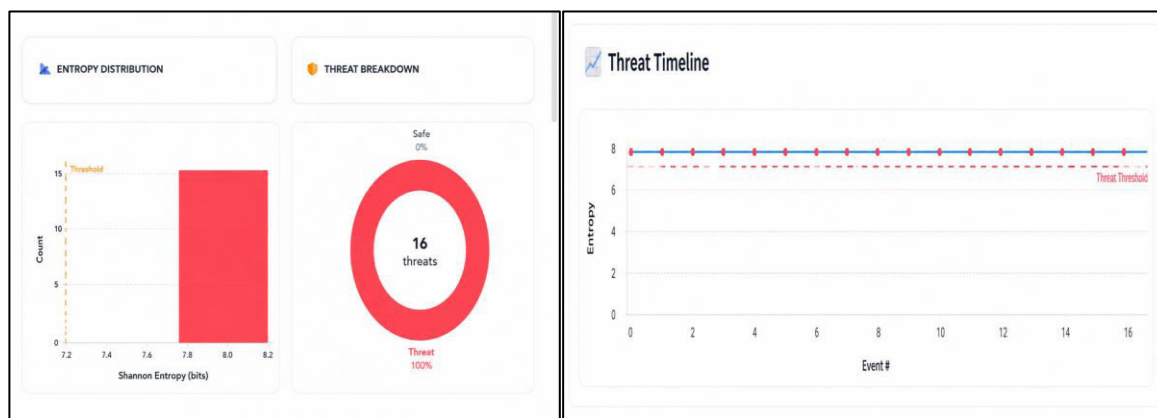
Fig.1. Entropy distribution and threat breakdown Fig.2. Entropy exceeds the predefined threat threshold
